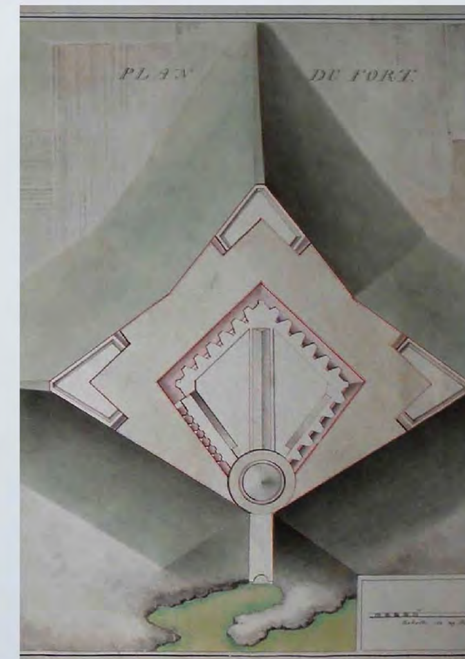
Details of the ground level (below) and terrace-level (above) plans of Fort Tigne from the original presentation drawing which shows the initial design concept. (Image source : Courtesy of the National Library of Malta). (Spiteri, 2011)
