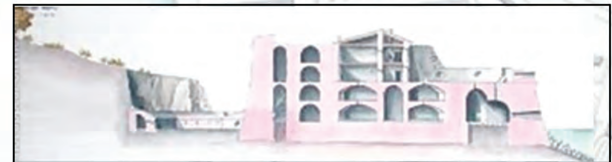
SECTION OF THE ROYAL TOWER REVEALS HOW THE WALL THICKNESS VARIES FROM 5 M TO 3 M, TO ACCOMODATE A CENTRAL CORE AND MILITARY-PRIORITIZED SPACES
